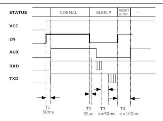
Figure 6: Timing diagram for Setting Parameters
