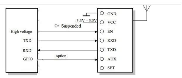
Figure 5: Connection diagram in circuit
