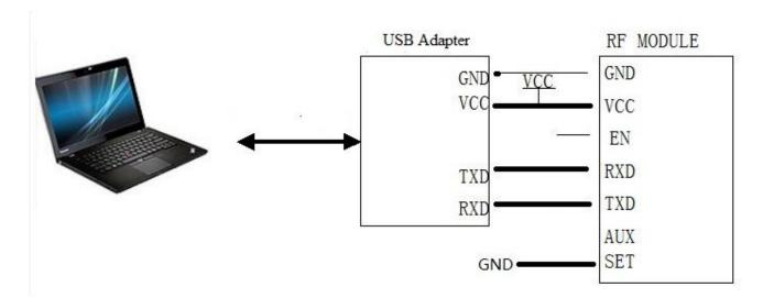
Figure 4: The connection diagram
