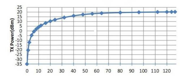
Figure 2: Indication of TX power level
