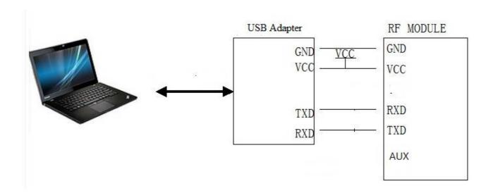
Figure 4: The connection diagram
