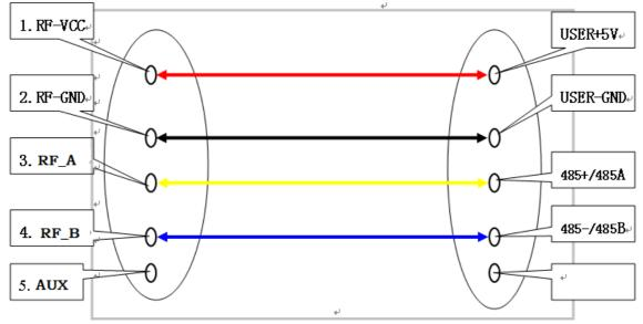
Figure 8: Connection between Module and Device(RS485 port)
