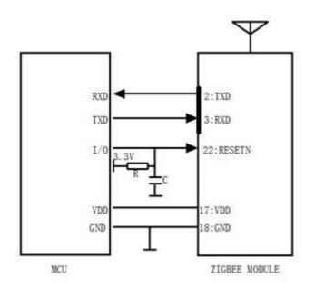
Figure 2: RF5168 Connection Diagram
