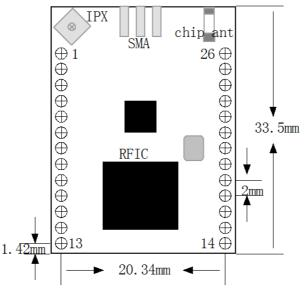
Figure 3: RF5168 Mechanical Dimension
