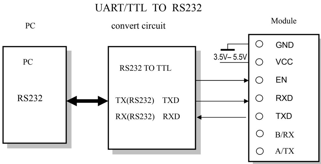
**Figure 3: The connection diagram**
