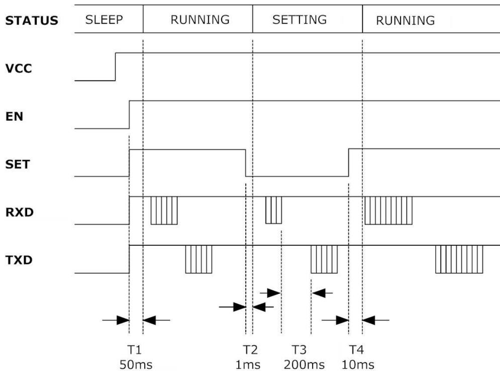
**Figure 4: Timing diagram for Setting Parameters**
