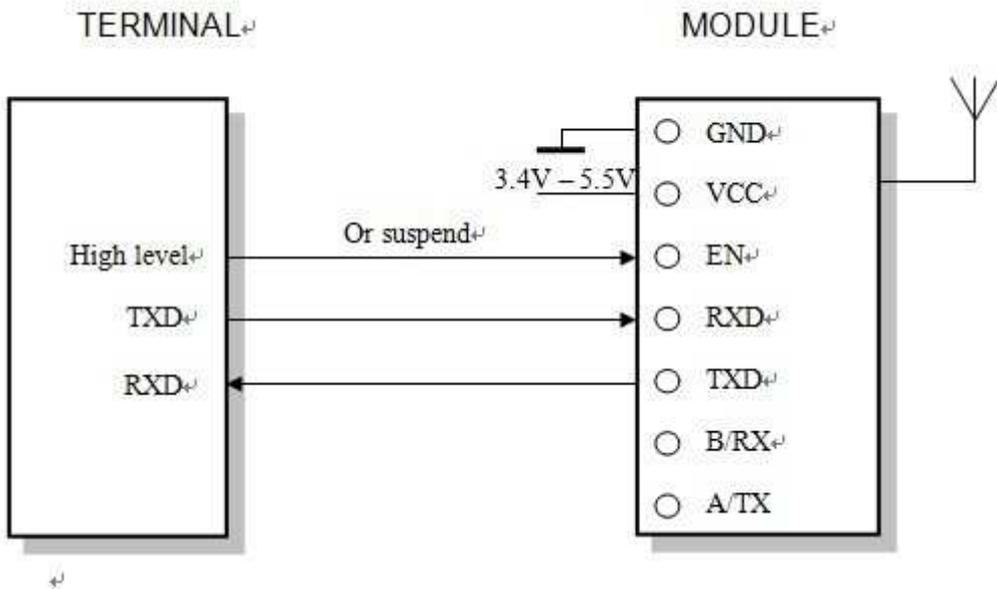
**Caution:** When RF7020-27 connect the UART/TTL interface, the B/RX&A/TX pin must be suspended.
