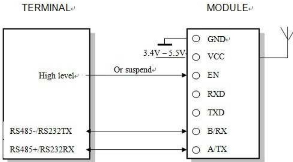
**Caution:** When RF7020-27 connect the RS485/RS232 interface, the TXD&RXD pin must be suspended.
