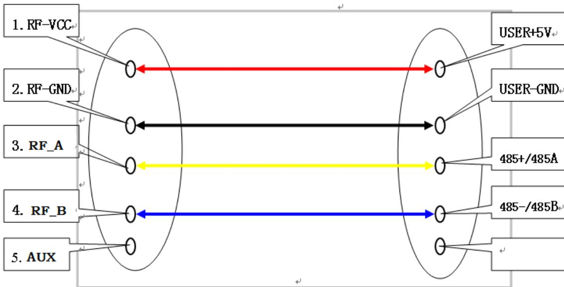
**Figure 8: Connection between Module and Device(RS485 port)**
